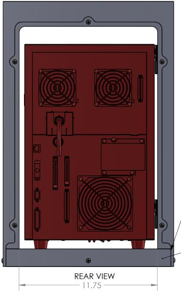
REMOVE SCREWS FROM REAR ACCESS PANEL REMOVE SCREWS FROM PERIMETER OF ENCLOSURE SLIDE ENCLOSURE FORWARD OFF BASE
