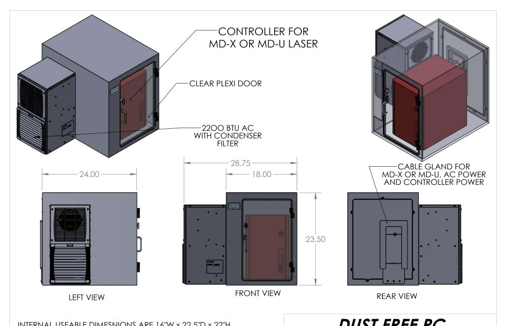
INTERNAL USEABLE DIMESNIONS ARE 16"W x 22.5"D x 22"H FRONT DOOR OPENING IS 12"W x 19"H REAR ACCESS PANEL OPENING IS 14.25"W x 19"H
