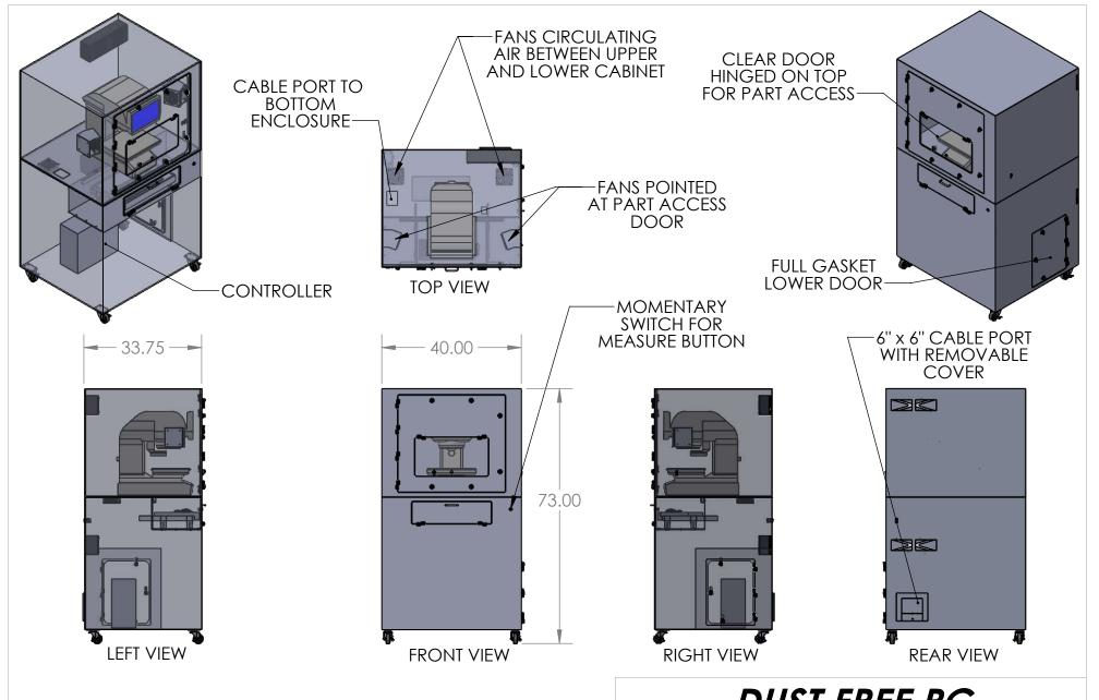
FRONT DOOR OPENING IS 30"W x 27"H PART ACCESS DOOR OPENING IS 21"W x 11.25"H LOWER CABINET SIDE DOOR OPENING IS 13"W x 18"H
